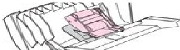
8. Make sure that both sides of the assembly are secured by the green hooks.
