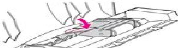
7. To check for proper installation, lift the green lever until it remains open. The pickup roller assembly should be secured to the lever assembly and should not fall out.
