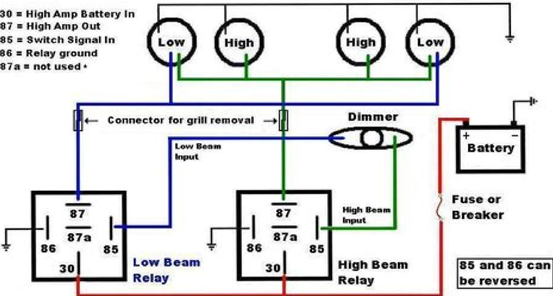
Headlamp harness should be upgraded to 14 ga wire throughout. OEM 1960 Chevy truck wiring shows 14 ga lt green for high beams, 18 ga tan for low beams, 20 ga black grounds!
