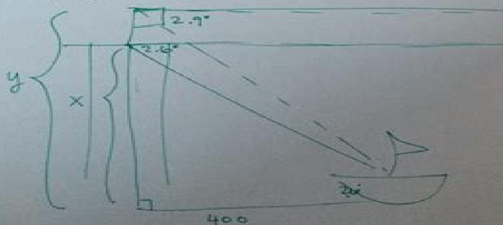
$$\begin{aligned}\tan 2.6 &= \frac{x}{400} \\ x &= 18.1639 \\ \tan 2.9 &= \frac{y}{400} \\ y &= 20.2631 \\ y - x &= 2 \text{ ft}\end{aligned}$$
