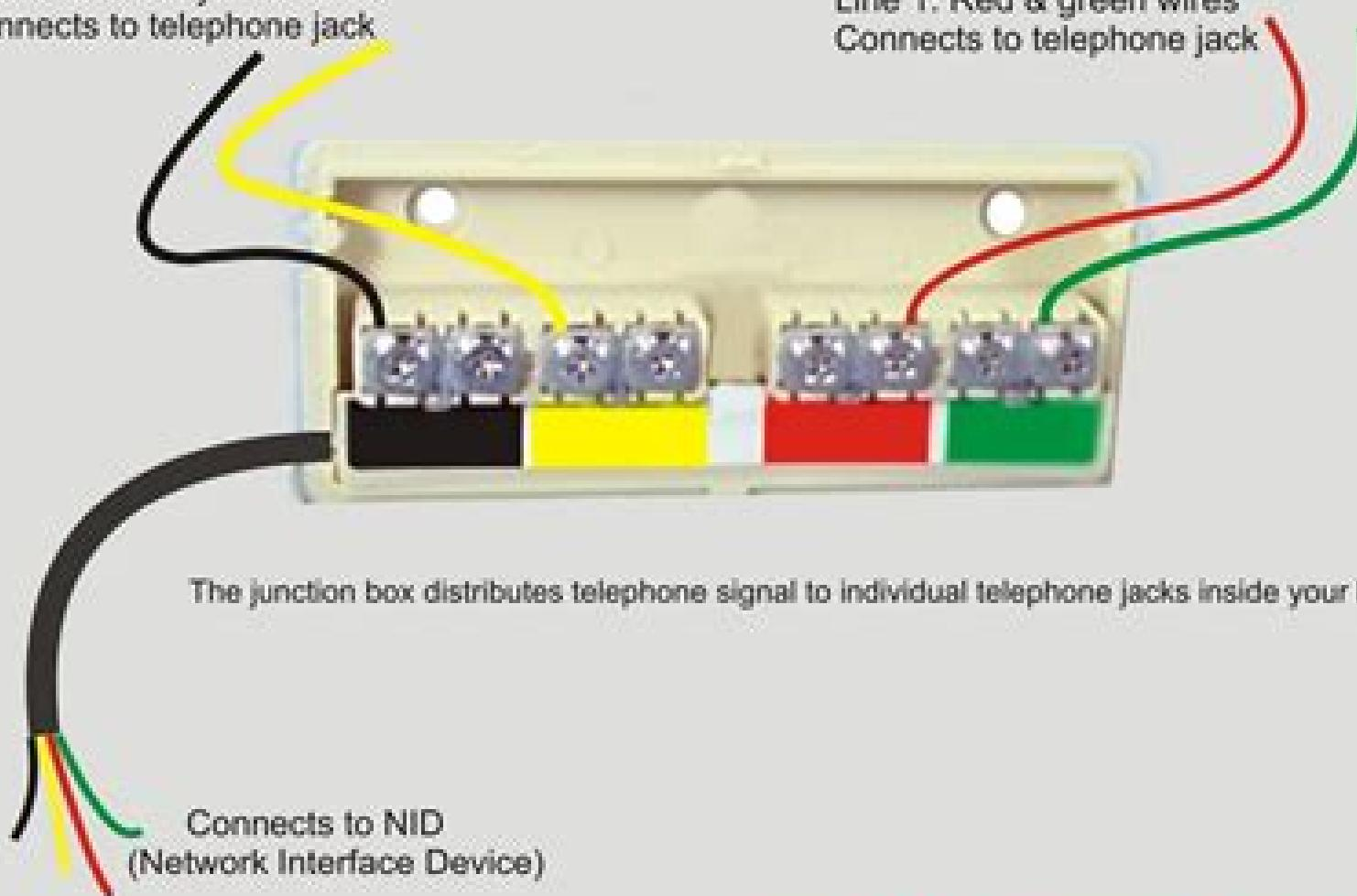
The junction box distributes telephone signal to individual telephone jacks inside your home.
