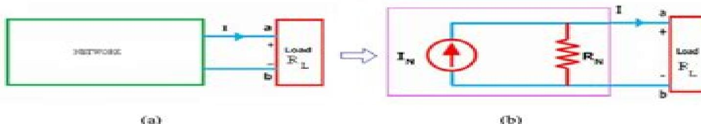
Figure (a) shows a simple block representation of a network with several active / passive elements with the load resistance  $R_L$  connected across the terminals 'a' and 'b' and figure (b) shows the Norton equivalent circuit with  $I_N$  connected across  $R_N$  and  $R_L$ .
