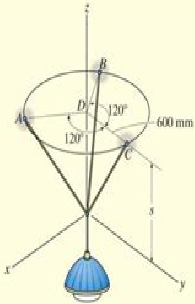
The 47.7-N lamp is suspended from 3 equal-length cords. Determine the smallest vertical distance of  $s$  if the force developed in any cord is not allowed to exceed 50N
