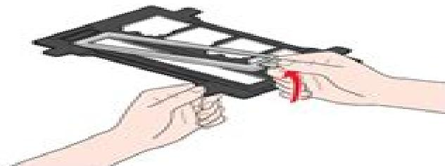
2. Slide your film strip all the way into the film holder with the shiny base side facing down. Your images and any wording on the film strip should appear backwards on the side that faces up. You can scan up to 6 standard 35mm images per film strip.
