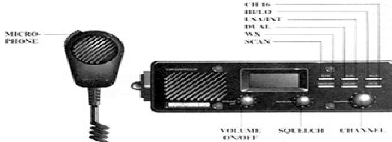
All features of your Humminbird VHF radio are controlled by the front panel knobs and buttons, plus the microphone button.
