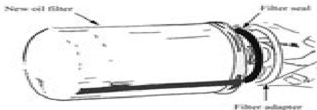
3. Clean any excess oil from filter and adaptor.
