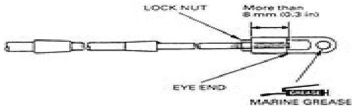
3. Install the shift cable by aligning the groove of the control cable with the cable guide plate.
