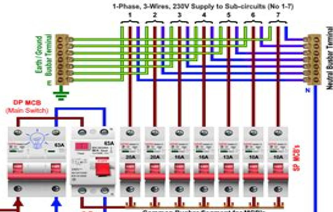
IEC & UK Wiring Colour Codes: 1-Φ, 230V
