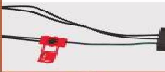
**2** Insert the connector wire (push the right sleeve) next to the other wires.
