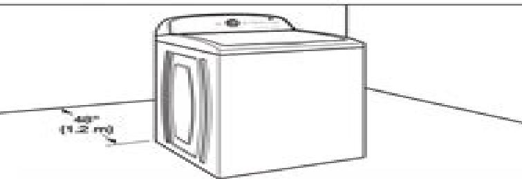
Move washer to within 4 ft (1.2 m) of its final location; it must be in a fully upright position.
