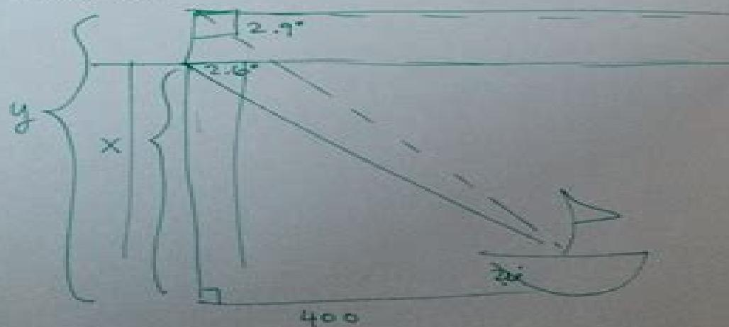
$$\begin{aligned}\tan 2.6 &= \frac{y}{400} \\ x &= 18.1639 \\ \tan 2.9 &= \frac{y}{400} \\ y &= 20.2631 \\ y - x &= 2 \text{ ft}\end{aligned}$$
