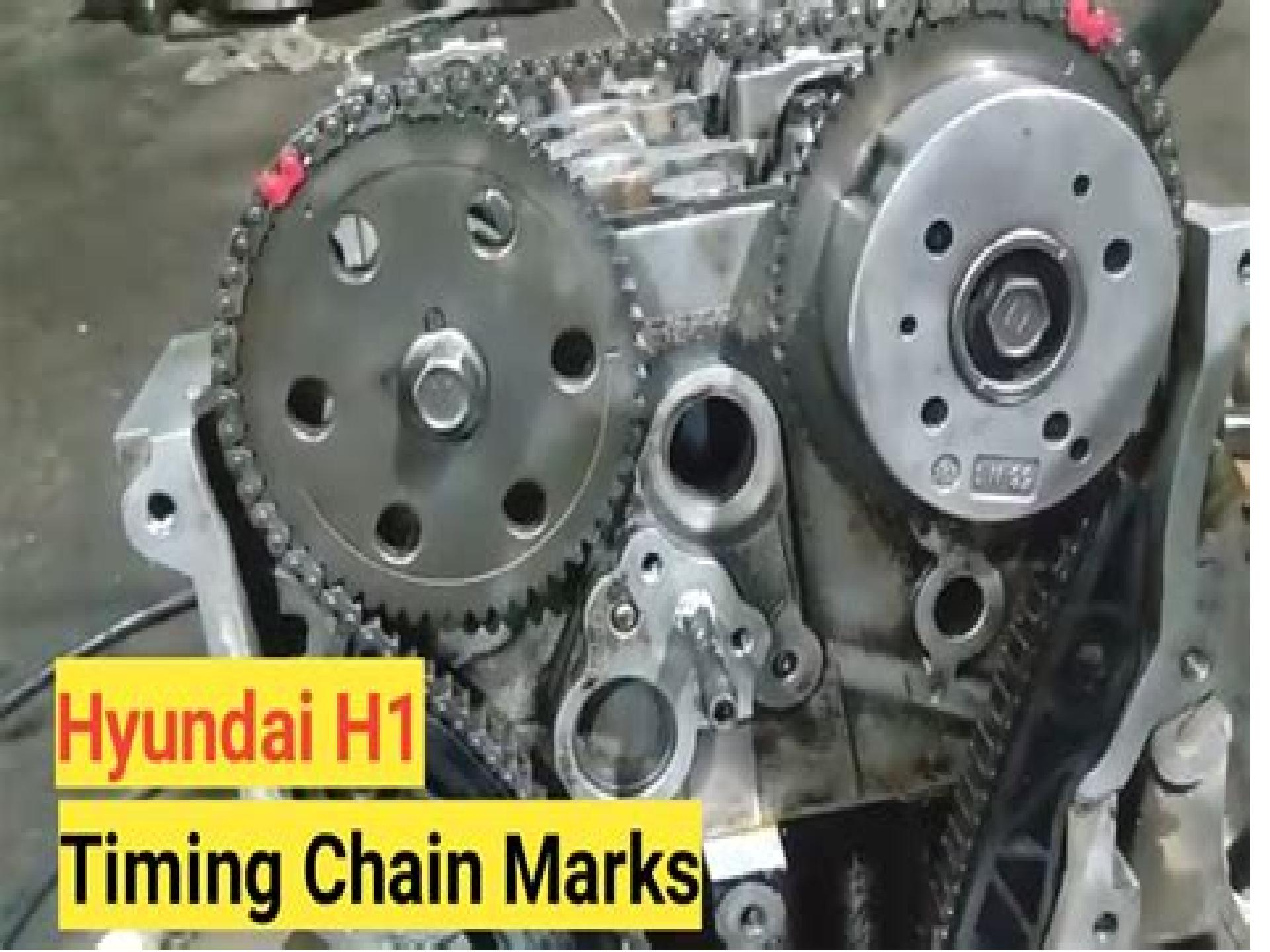
A close-up photograph of a car engine's timing system. The image shows a timing chain with several sprockets and tensioners. The engine block is visible in the background. The text 'Hyundai H1' is overlaid in a yellow box on the left, and 'Timing Chain Marks' is overlaid in a yellow box at the bottom left.
