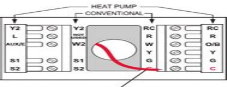
For 24VAC primary power, connect common side of transformer to "C" terminal.
