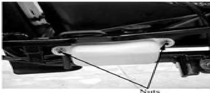
Open the reserve tank cap and drain the coolant from the reserve tank.
