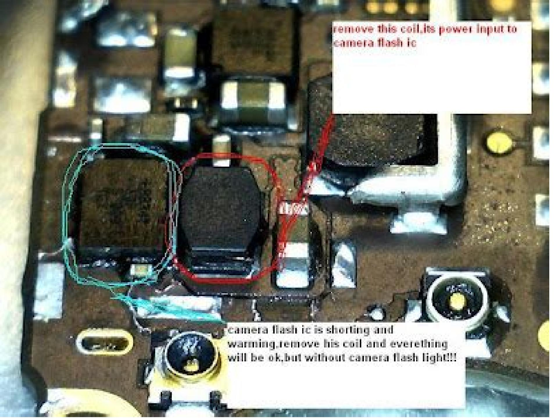
remove this coil,its power input to camera flash ic
