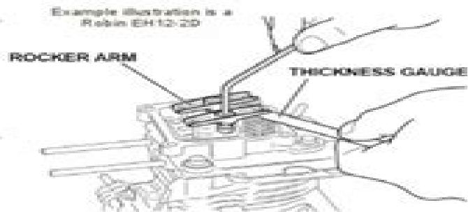
**NOTE:** Always check and adjust valve clearance while engine is cold
