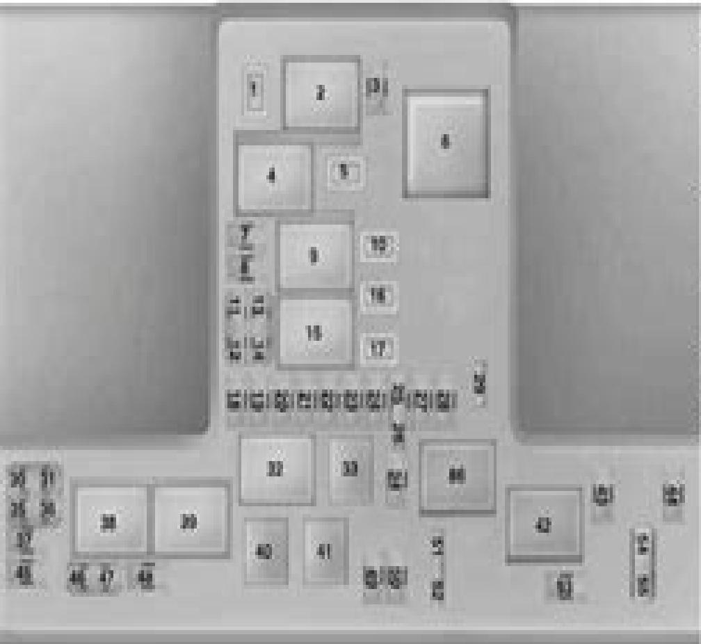
The power distribution box is located in the engine compartment. It has high-current fuses that protect your vehicle's main electrical systems from overloads.
